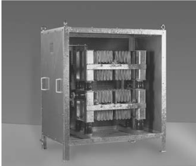
Figure 13.11 Earthing resistor made from meandering wire for outdoor installation 16 \Omega , 400 A for 10 s, 75 kV BIL, IP 20
