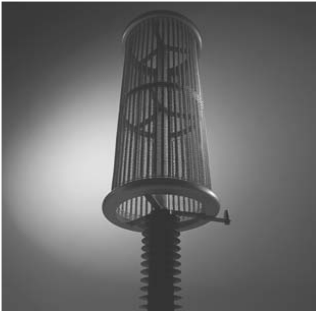
Figure 13.10 Earthing resistor made from CrNi-alloy steel fabric for indoor installation 3810 \Omega , 5 A for 10 s, 170 kV BIL, IP 00
