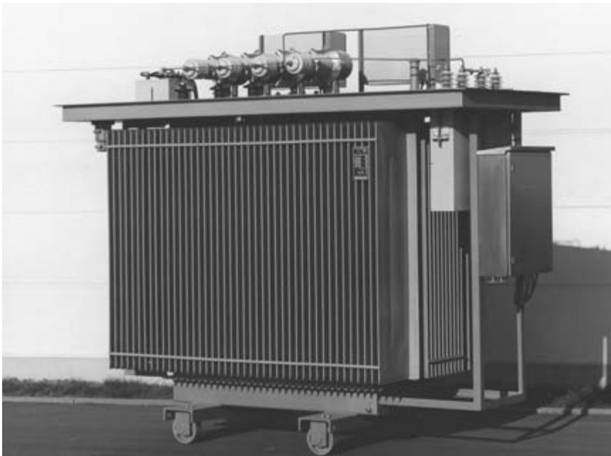
Figure 13.9 Adjustable Petersen-coil 21 \text{ kV}/\sqrt{3} ; 4 \text{ MVar} ; I_r = 70.1\text{--}330 \text{ A} ; adjustable in 64 steps, 4.13 \text{ A} each
